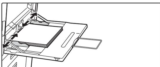
Set the bypass tray guides correctly to the width of the paper.
