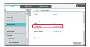
Check the IP address in the machine information
