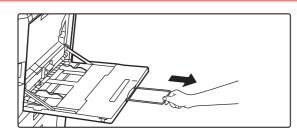
When loading paper larger than A4R or 8-1/2 x 11R, pull out the extension guide.
